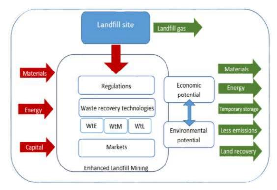
Figure 1: Landfill mining and ELFM process
