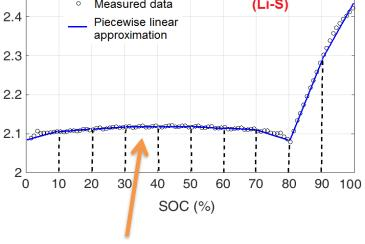
Flat 'low plateau' makes it impossible to estimate remaining capacity from open-circuit voltage alone.
