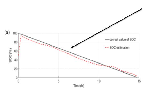
ANFIS together with current integral gives mean error ~4% with UDDS automotive cycle.
