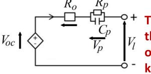
This is potentially more useful, but the challenge here is that the load voltage depends on the current so we can only calculate it after the event – unless the current is known in advance.
