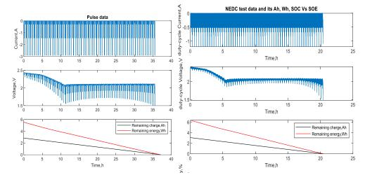
$\overline{E}_{\ell} = \int_{\text{discharge}} V_{\ell} I_{\ell} dt$
