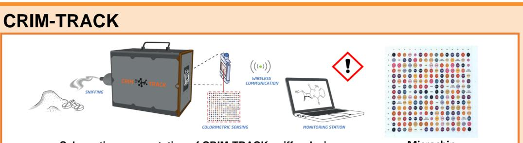
Schematic representation of CRIM-TRACK sniffer device.
