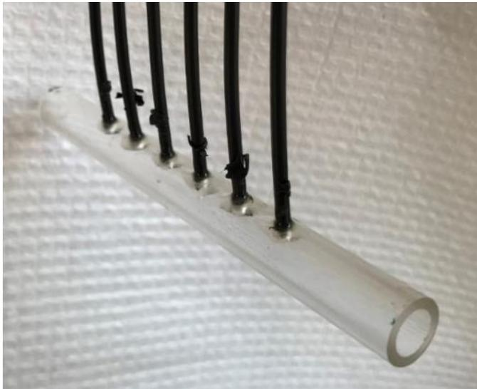
**Figure 14.** Photograph of an assembled burn tube. Tube has a 5 or 7 mm internal diameter and 100 mm in length. 6 ports are drilled into the tube that are 10 mm apart, fibre optics are fitted into the holes and secured with a 5 minute cure two part epoxy.
