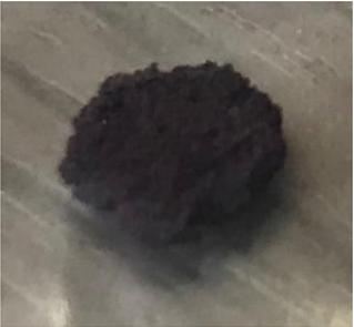
**Figure 23.** Printed thermite disc.
