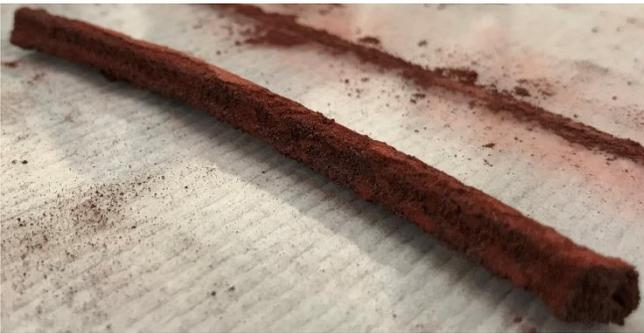
**Figure 24.** Printed thermite cylinder.
