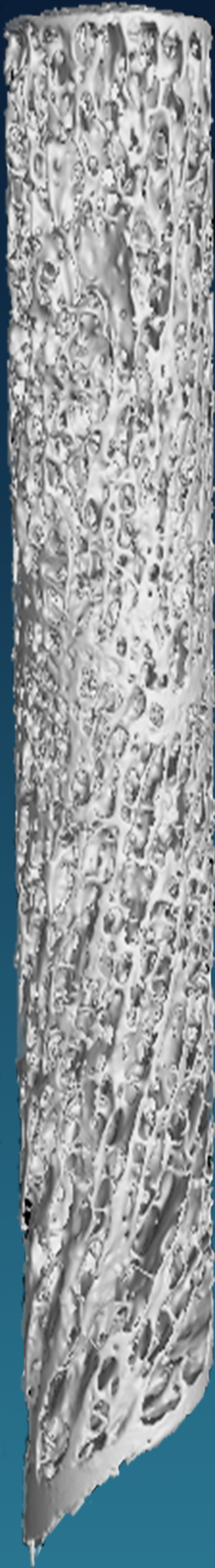
Figure 1: Sample \mu CT reconstruction image of femoral core
