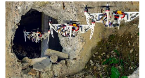
Multi-drone system flying into a potentially unsafe environment (Search and Rescue) Robotics and Perception Group, ETH Zürich. http://rpg.ifi.uzh.ch/
