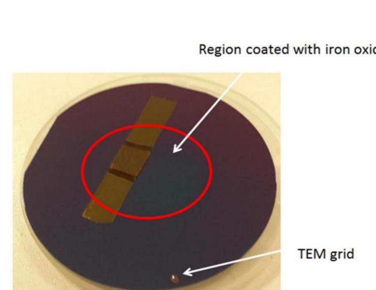
Fig. 5:  $\text{Fe}_3\text{O}_4$  coating in centre of silicon wafer.
