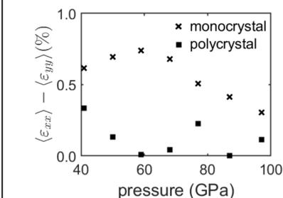
**Fig. 7:** Difference between the two transverse components of elastic strain as a function of pressure for the monocrystal and the polycrystal.
