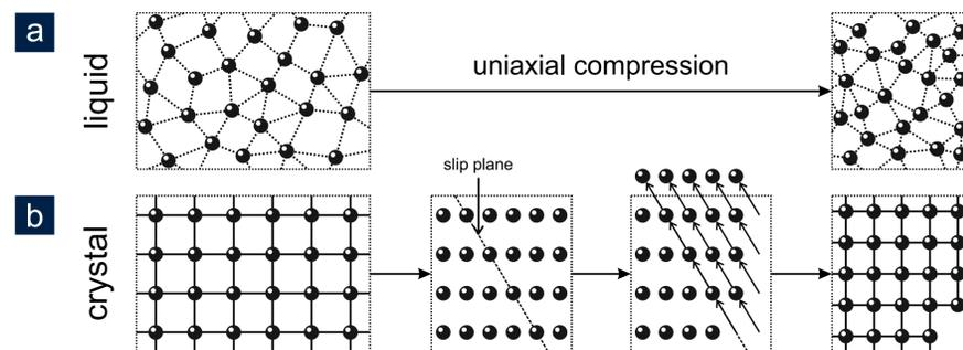
**Fig. 3:** Schematic depiction of (a) a liquid and (b) a crystal responding to uniaxial compression.
