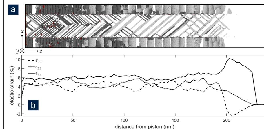
**Fig. 5:** Response of polycrystal shock-loaded along the z-direction to 40 GPa. (a) Atoms located in proximity to slip or twin planes. White and grey atoms experience relative motion in the xz-plane, red in the xy-plane. (b) Elastic strains along the x-, y-, and z-directions as a function of distance along the crystal. The strain quantifies how closely spaced atomic planes are in each direction.
