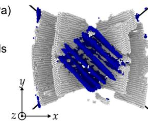
**Fig. 6:** transverse twinning in a grain in a polycrystal shocked to 60 GPa.
